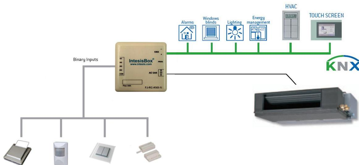
FJ-RC-KNX-1i allows a complete and natural integration of Fujitsu air conditioners with KNX control systems.
