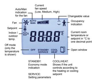
The display is handled using the buttons on the controller:
